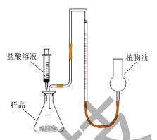
图 1 充气硬糖中气体在常压下体积的测定装置 Fig.1 Device for volume determination of CO<sub>2</sub> gas of popping candy at normal pressure
