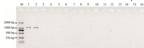
Fig. 2. Agarose (1%) gel electrophoresis of PCR products amplified using primers Outer F and Outer R
