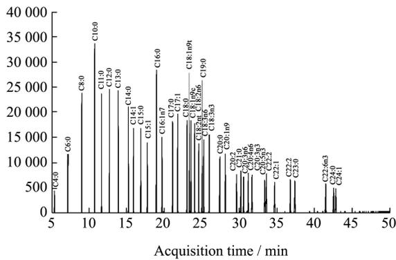
Fig.1 TIC diagram of 38 fatty acids mixed specimens including internal standard for separation
