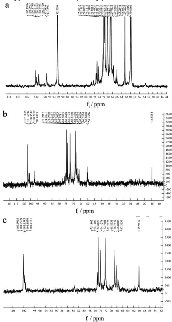
Fig.3 The <sup>13</sup>C NMR spectra of the polysaccharide fractions: (a) TM-P1A; (b) TM-P2A; (c) TM-P2B
