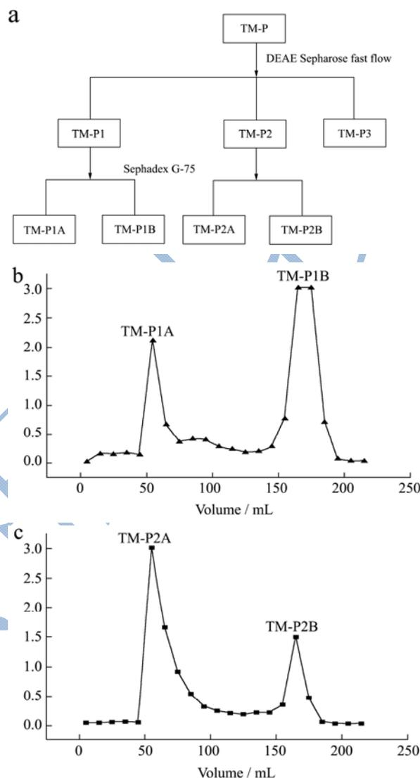
Fig.1 Scheme of purification of crude TM-P (a) and elution curve of polysaccharide fractions (TM-P1 and TM-P2) on size-exclusion chromatography column of Sephadex G-75 (b and c)
